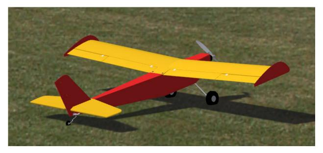
The electric drive is considerably stronger than the .19 engine with the small propeller. The model climbs much better and is faster, all setup parameters still the same. There are only two concessions to the bigger power and agility: To have adequate roll agility, aileron throw is set to 20° (instead of 15°). And since landings are faster, flap deflection is 45° (instead of 30°).
