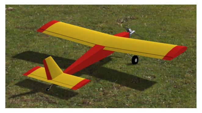
The model now weighs another 200 g / 7 oz more to allow for ailerons, servos, and linkages. The thrust/weight ratio is further reduced to 0.52 what you still won't really notice as well as the higher wing loading.
