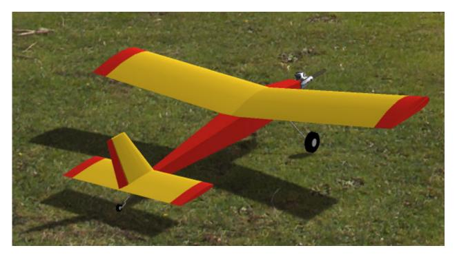
This is the model as I had it in reality. The square 5:1 wing has 6 degrees dihedral, which is rather little for a rudder-and-throttle model as is the 2 degrees decalage. Together with the wing's airfoil and aspect ratio and the model's weight, this makes for a calm and sluggish flight behavior even in gusty wind. And it's just sufficient to control the model with its low-aspect-ratio wing.
