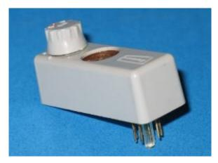
Look at this elaborate plug and socket! They were used for all connections of the radio's airborne components. The male plug had eight gold-plated contact pins arranged in a circle around a central key pin, the female plug the corresponding eight gold-plated contacts around a central hole with a slot. So all connections were polarized and electrically safe what contributed to the radio's reliability.
