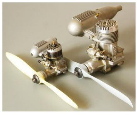
That is 1.3 times the power of an older .60 of the 1960s (for instance the O.S. "Gold Head") and 4.5 times as powerful as the old .19 engine.
