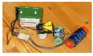
Each stack of cells was wrapped in transparent-blue heat-shrink tube and had one clip at each end. It was the sort of clips known from the 9V monobloc batteries, a male one at one end (+) and a female one at the other (-). So they were polarized, and the corresponding colored clips on the cable could not be plugged the wrong way.
