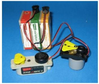
The green and orange boxes are 2-channel "switching" modules, corresponding to the transmitter stick movements left/right (green) and fore/aft (orange). Each module contained two transistorized tone filters (a Schumacher invention) and two relays. The receivers didn't have "reed banks" like those of other brands and didn't need any finetuning to the transmitter. That was a unique feature and made these sets very reliable. The <u>stack</u> of boxes was put into the model's
